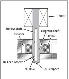
prevents bearing temperature increases, and offers high reliability. In addition, the specially treated shaft journal keeps the bearing from being damaged during high temperature operation.
