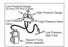
4) Leave the high pressure valve and the lowpressure valve of the gauge manifold closed for five min or more, and confirm that the gauge pointer does not return to zero.
