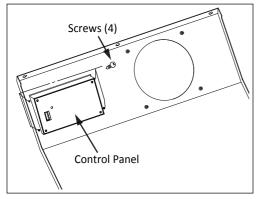
1) Take out the four (4) screws, and then remove the control panel.
