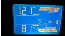
We recently did some testing of small UPS. These were the Orion Online RT, the Orion Office Pro and the APC SmartUPS. We varied input voltage to each UPS to test voltage regulation in normal operation and to determine when they transfer to battery.
