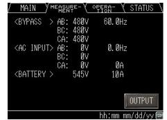
Figure 4-13 Measurement screen (Battery Operation)
