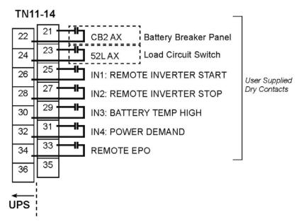
Figure 4-17 External Signal Terminal Block TN11-14 (NEC Class2)
