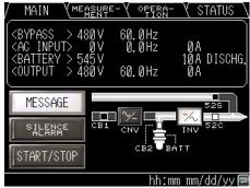
Figure 4-14 Main screen (Fault indication)
