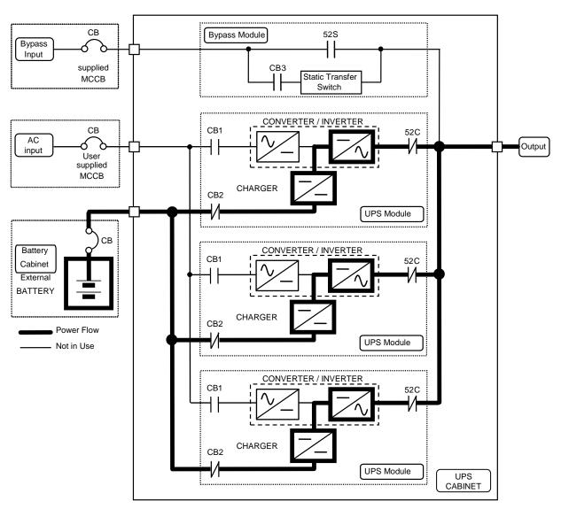
Figure 2-3 Single Line Diagram - Battery Operation
