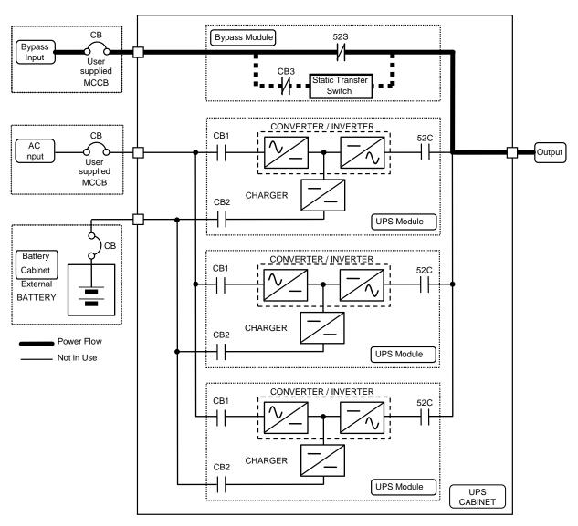
Figure 2-2 Single Line Diagram - Bypass Operation: Load fed through static bypass line
