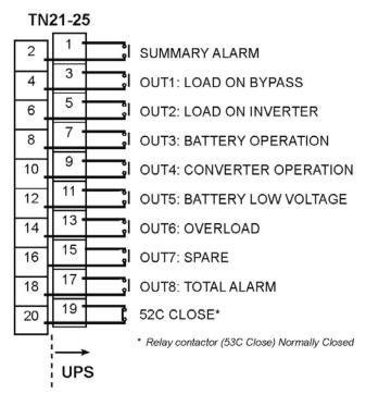
Figure 4-16 External Signal Terminal Block TN21-25 (NEC Class2)
