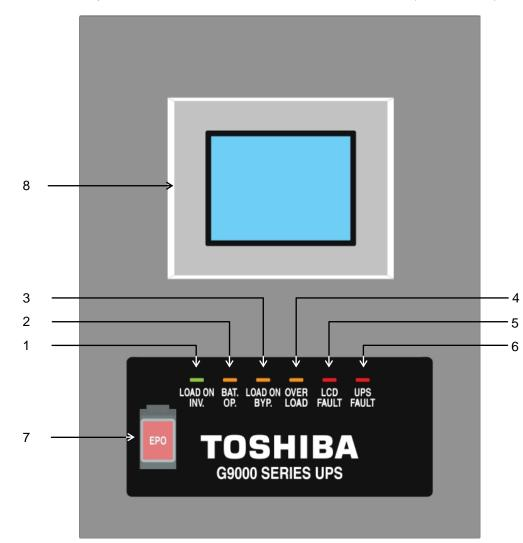
Figure 4-1 Operation/Display Panel (Front panel)
