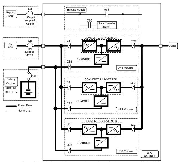
Figure 2-1 Single Line Diagram - Normal Operation: Load powered by UPS inverter
