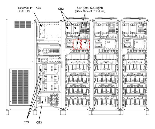
Figure 2-5 UPS Parts Location – Front Inside View
