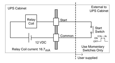
Figure 4-19 Remote "Start" Contact Connections
