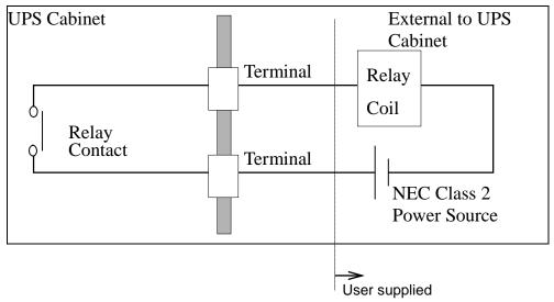
Figure 4-18 Control Wiring for External Contacts
