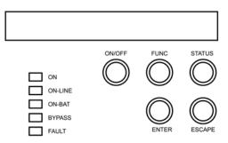
Figure 4 Control panel – 2400VA Tower/6000VA Rack Unit
