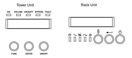
Figure 3 Control panels – 1000/1500/2000/3000VA
