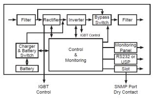
Figure 1. Block diagram
